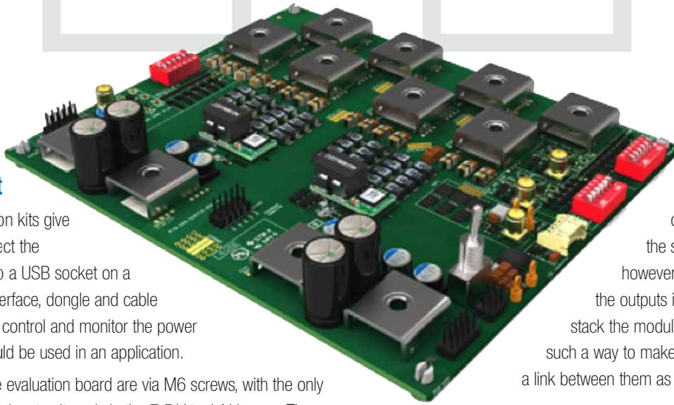
output connections use the same M6 screws, however, if you want to connect the outputs in parallel or you wish to stack the modules, they are placed in such a way to make the operation of placing a link between them as easy as possible.
