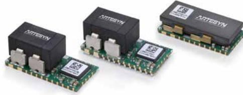
used for power conversion. This is now also true of the total volume of the power-conversion stages, and so module height is also under pressure to be reduced. The low-profile version of the LGA50D addresses this and has one of the highest power densities in terms of Amps per cubic inch on the market for this type of power converter. LGA50D has also been designed with cost in mind to address this key factor in decision making of a power conversion solution.
